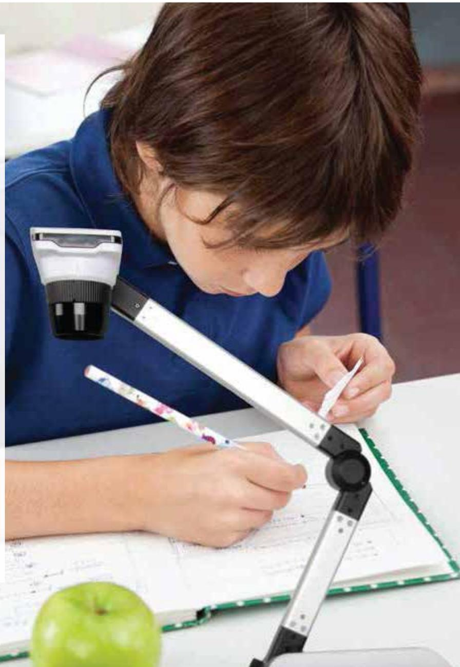
The new DC2L document camera is capable of delivering incredible high image quality with its 8MP camera, direct HDMI output at 30fps, full A3 shooting area, and 17x optical zoom.
